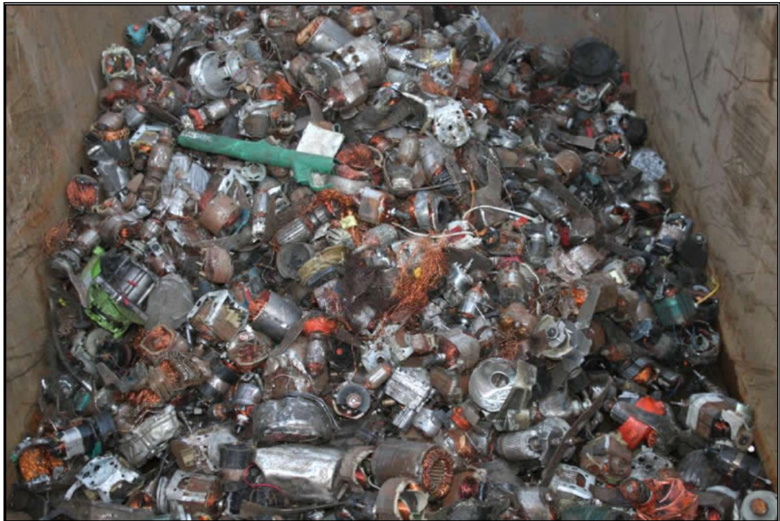
Picture 15 : Category 6 motors made a significant contribution the overall metal content for this category.
