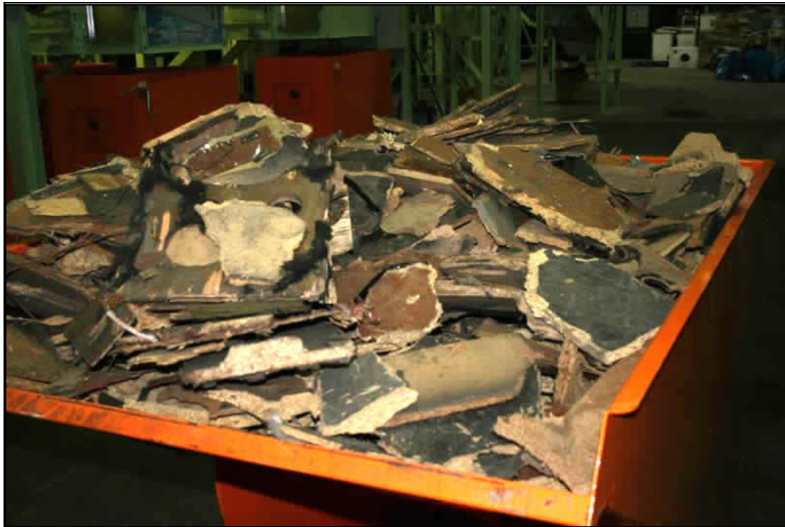
Picture 13 : Category 4 Segregated wood and chip board materials. Derived principally from speaker and stereo cases.
