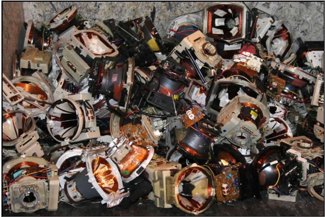
Picture 19 : CRT Dismantling. Yolks collected from category 3 PC Monitors. Samples of these were collected and hand dismantled to determine composition.
