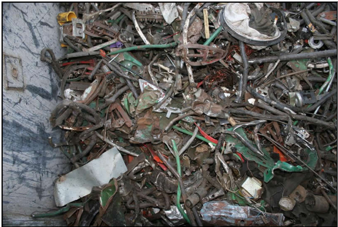
Picture 16 : Category 6 Ferrous. The majority of this fraction was made up of handles, metal body panels and other non motor components.
