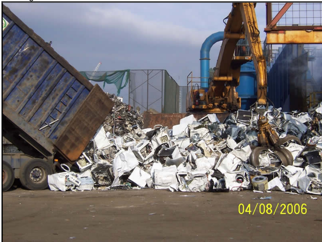
Picture 2 : 109 Tonne sample of large category 1 items. Loading in to shredder.
