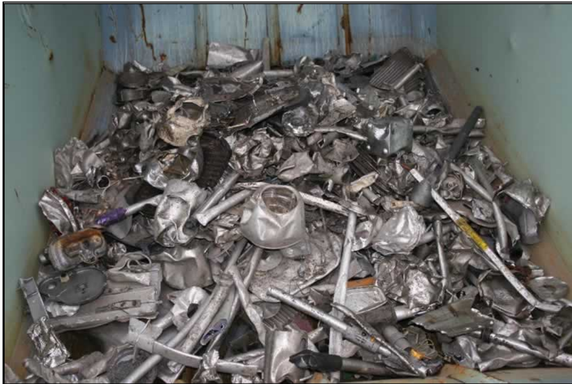
Picture 5 : Category 2 'non-ferrous' (including some stainless steel) output. Vacuum cleaner pipes, toaster/grill plates and kettles were present.
