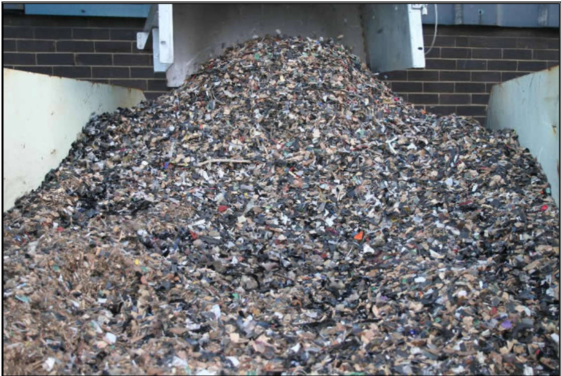
Picture 11 : Category 4 Plastic rich output. Representative samples of this material were taken to handsort. There was a significant wood component to this material.
