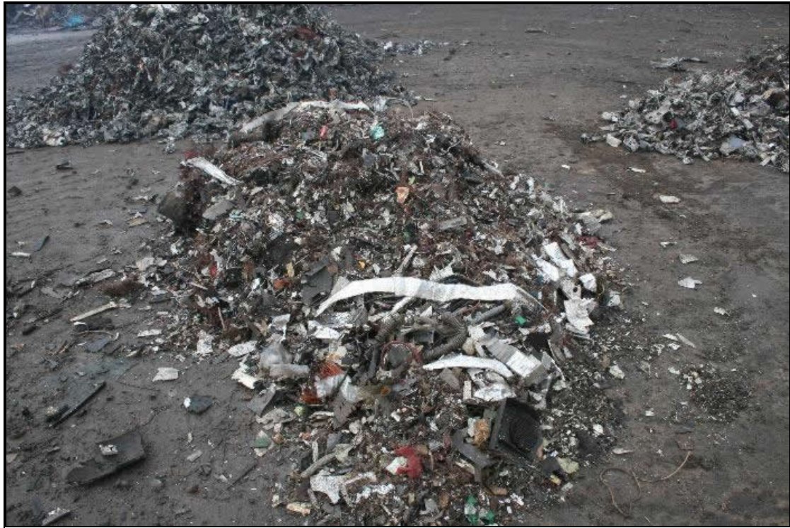
Picture 21 : Category 1 small household appliances. This is the 'frag dirt' (near centre), and shredder non ferrous (rear right), from shredding 9.2 tonnes of small category 1 items, including microwaves, heaters and fans. These materials were sampled. The representative samples were then handsorted to determine metal, plastic and other material content.
