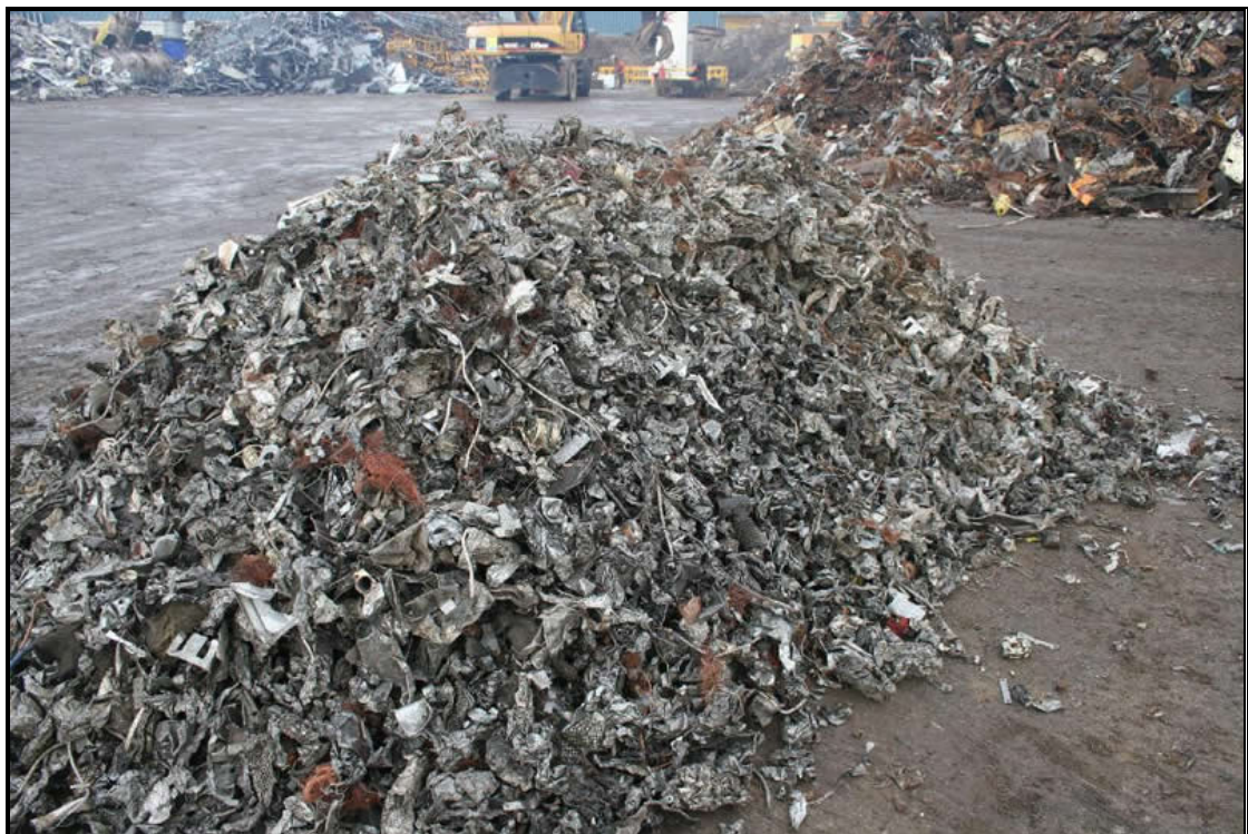
Picture 20 : Category 1 small household appliances. This is the Ferrous product (3a-3b) from shredding 9.2 tonnes of small category 1 items, including microwaves, heaters and fans.
