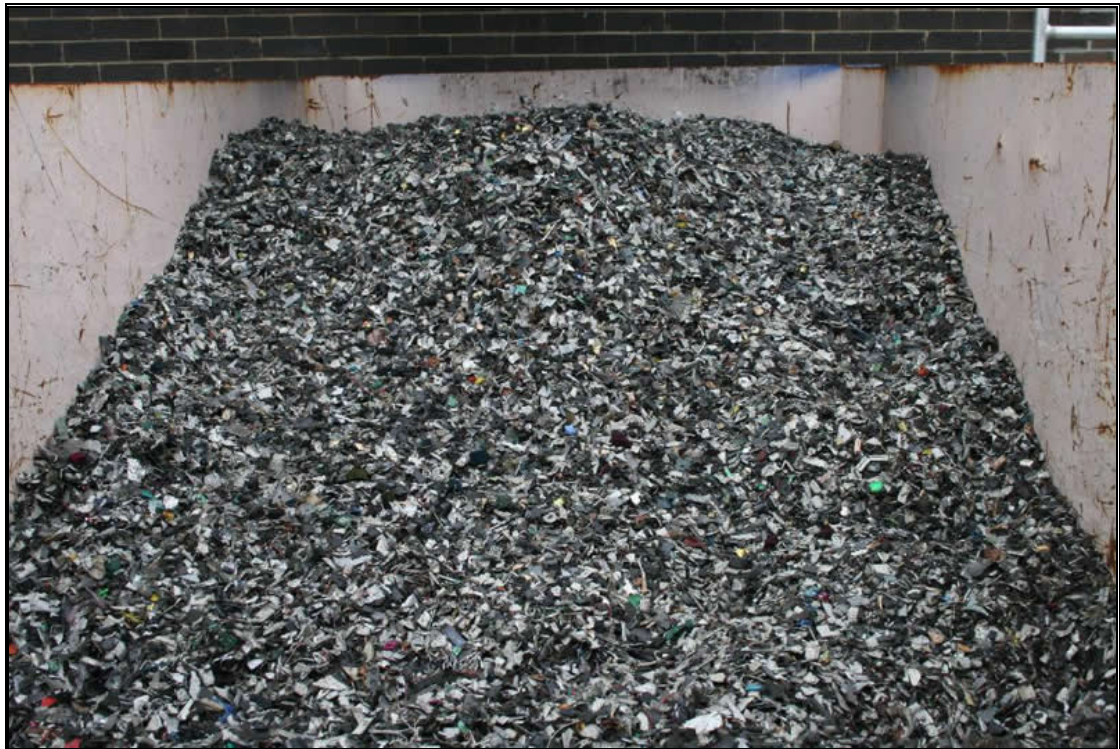
Picture 7 : Category 3 plastic dominated output. Representative samples were taken for handsorting to determine composition. The output was dominated by grey and black plastics.
