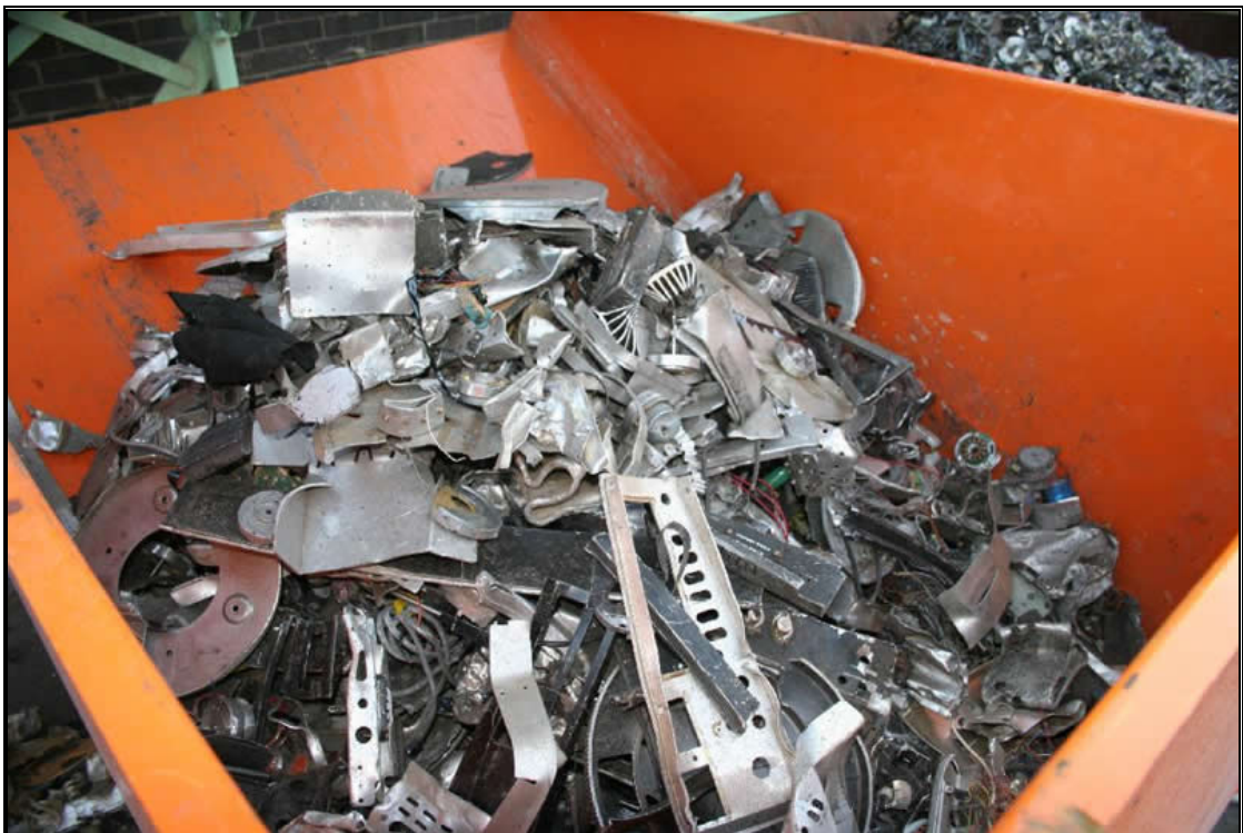
Picture 12 : Category 4 Non ferrous output. Other non ferrous materials appeared within a granulated output.
