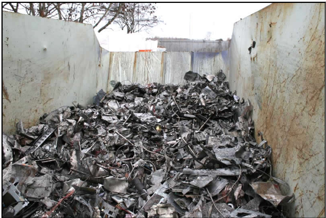
Picture 7 : Category 3 plastic dominated output. Representative samples were taken for handsorting to determine composition. The output was dominated by grey and black plastics.
