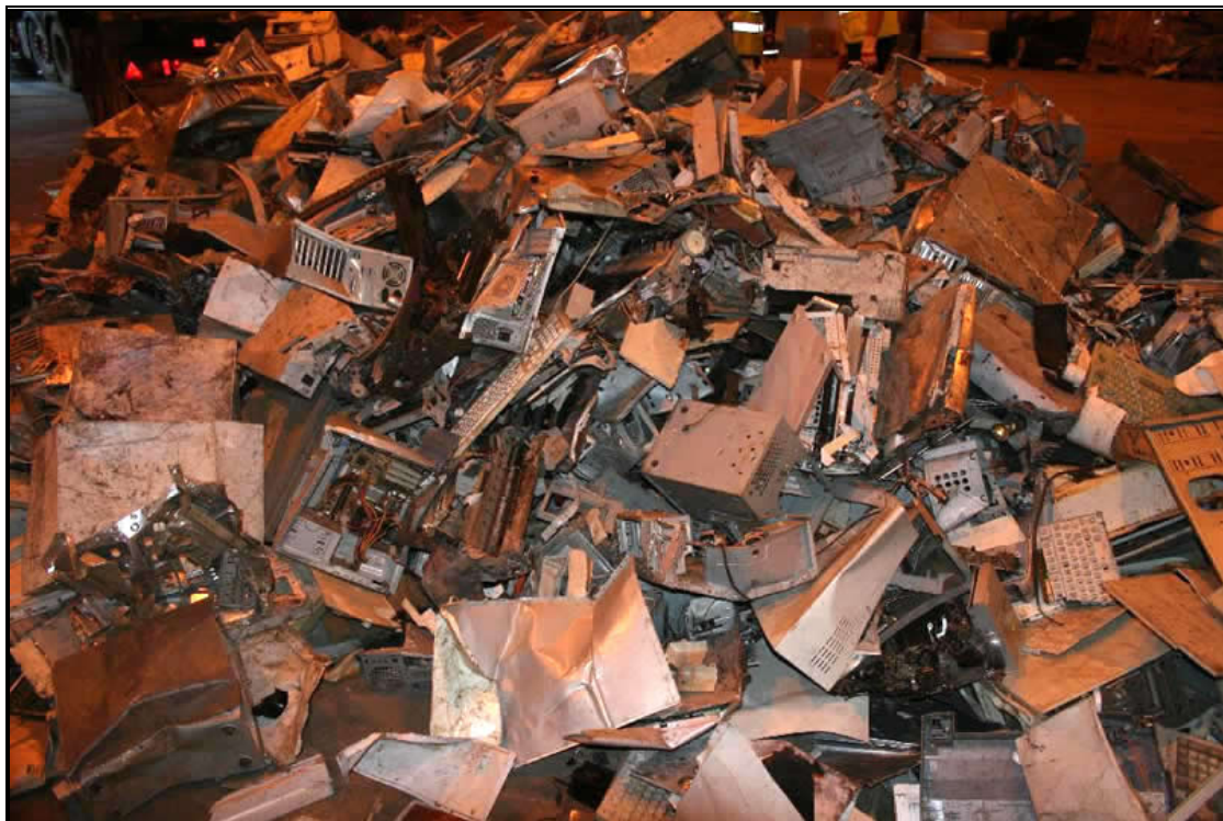
Picture 5 : Category 2 'non-ferrous' (including some stainless steel) output. Vacuum cleaner pipes, toaster/grill plates and kettles were present.
